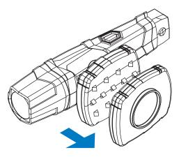
The magnetic clip is designed to allow some rotation up or down, so you can adjust the camera's angle after it is mounted.
