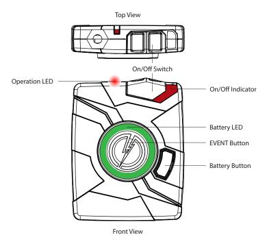
1 Operation LED – Shows the controller's current operating mode:
