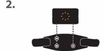
Snap Zeo pod on to sensor pad.
