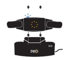
Lift headband off dock. Blue light will start flashing. Headband is now discoverable. (If the blue light stops flashing before you have completed step 5, press and hold headband button for 3 seconds until blue light is flashing.)
