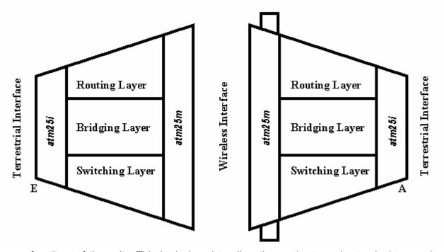
functions of the unit. This is designed to allow the reader to understand where an incoming service is terminating and where its configuration is managed. Management files (on Flashfs) for each layer are as follows:
