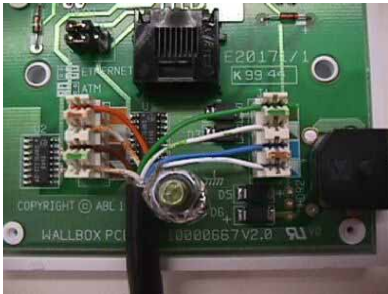
Figure 5-12 Interconnect Cable Connections to Indoor Junction Box
