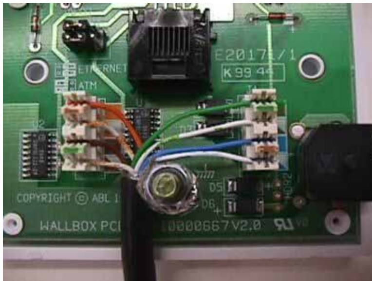
Figure 6-12 Interconnect Cable Connections to Indoor Junction Box
