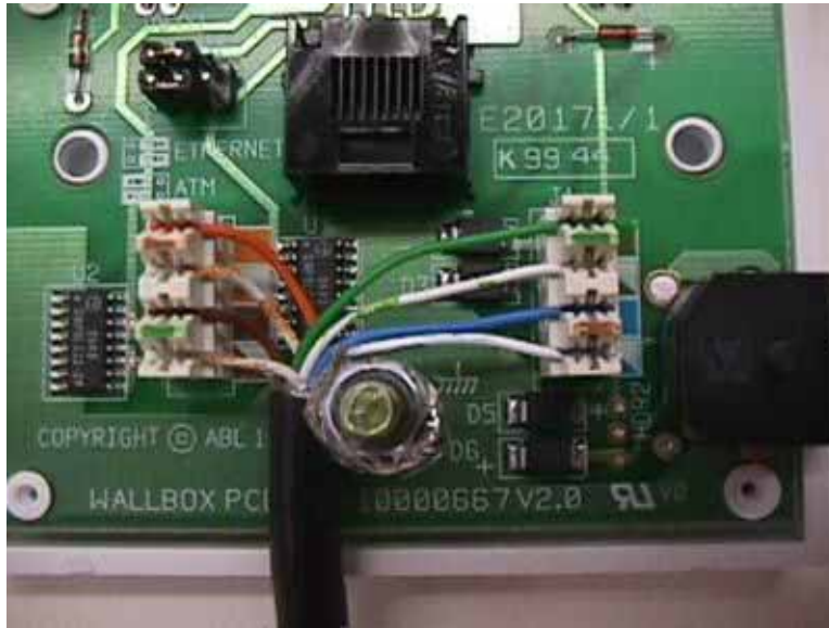
Figure 4-13 Interconnect Cable Connections to Indoor Junction Box
