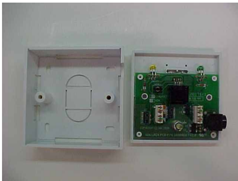
Figure 7-1 Indoor Junction Box (Wall Plate Enclosure)
