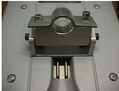
Figure 5-5 Access Point with Mounted Tilt Bracket
