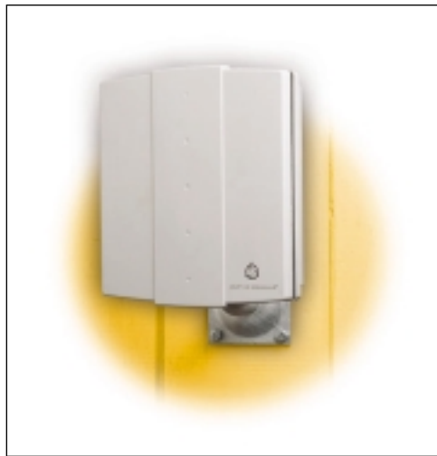
Figure 7-6 Outdoor Subscriber Unit Mounted on Wall
