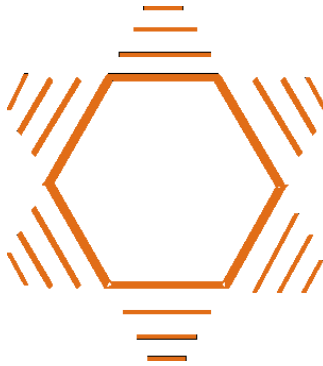
Figure 5-1 Diagram of Six Access Points for 360 degree Coverage
