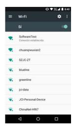
Touch Settings> WI-FI. Check Wi-Fi to turn it on. The phone scans for available Wi-Fi networks and displays the names of those it finds. Secured networks are indicated with a Lock icon.
