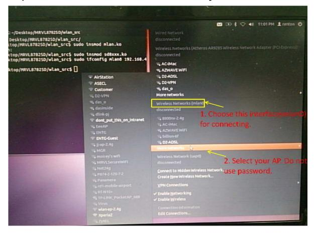
You can do further RF set up by using command "iwconfig".
