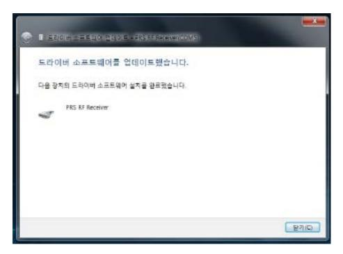
After completing installation, Device Manager/Other Device/PRS RF Receiver is Device Manager/Port(COM & LPT)/ PRS RF Receiver(COM5).
