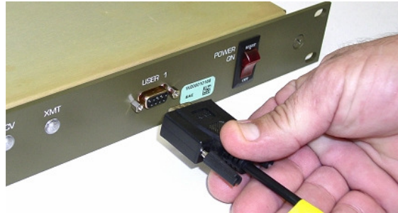
Figure 9. 1UR User Port Connection
