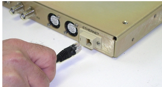
Figure 7. 1UR AX100617-00x Network Connection
