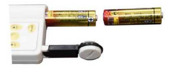
As shown in the upper right phote, put two AA alkaline batteries in the battery case. Make sure the plus side of batteries (convex) comes to the cap side.
