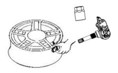
1.3 Take off the nut 5, insert the valve stem through the rim hole from inside.
