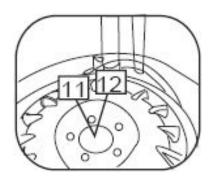
2.3 Use the same procedure to dismount the lower tyre bead. (If the mounting head of the tyre changer is at the 12 o'clock position, then the valves stem should also be at the 12 o'clock position.)
