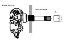
1.4 Place nut 5 on the valve stem, and tighten with 5 Nm (44 inch pounds) torque.
