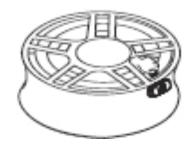
1.5 Lock the rim on the tyre changer. (If the mounting head of the tyre changer is positioned at 12 o'clock, then the valve should be at the 7 o'clock position.) Apply lubricant on both the tyre bead and rim. Mount the lower tyre bead on the rim. Ensure that the tyre bead does not touch the electronic module during mounting.
