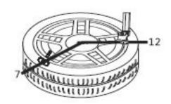
1.6 Mount the upper tyre bead the same way. (If the mounting head of the tyre changer is positioned at 12 o'clock, then the valve should be at the 5 o'clock position.) Inflate the tyre to nominal pressure.
