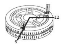
1.7 Apply soapsuds on the valve tip. If no leakage is found, put on the valve cap<sup>6</sup>. If unsuccessful, try again.
