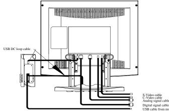
Analog signal cable Digital signal cable (DVI) USB cable from monitor to PC
