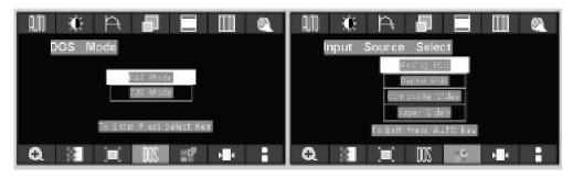
Push "Up" or "Down" button to select between "640 Push "Up" or "Down" button to select between Mode" or "720 Mode" "Analog RGB", "Digital RGB", "Composite Vid
