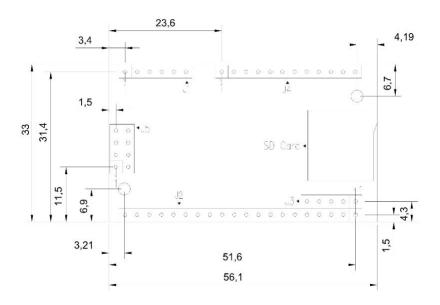
The above drawing shows the component side which faces down onto the carrier PCB.
