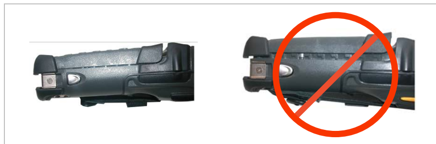
Figure: Keypad mounted correctly
