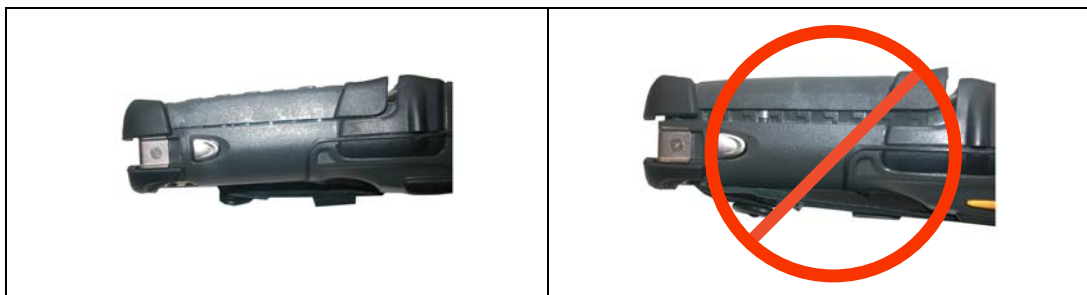
Figure 5: Keypad mounted incorrectly
