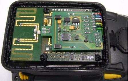
A photograph showing a green printed circuit board (PCB) with various electronic components, including a large chip and several connectors, mounted inside a black plastic housing. The board is secured with yellow wires. | <p>Insert the UHF reader into the upper housing.<br/>Solder appropriate wires on the UHF board as shown in the picture and fix them with UV-glue.<br/>Apply Sikaflex in the sealing area of the housing.</p> |
