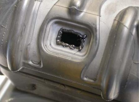
A close-up photograph of the grey plastic housing, showing a square opening in the center. The opening is filled with a dark, viscous substance, likely resin or Sikaflex, used for sealing.                              | <p>Fill the resin into the RFID housing (without empty space) and apply the opening of the lower housing with Sikaflex</p>                                                                                   |
