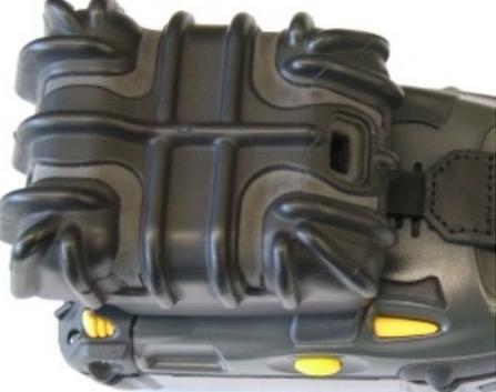
A photograph of a grey plastic component, identified as the RFID lower housing, which has a complex, multi-lobed shape with several protrusions and recesses.                                                              | <p>Put the RFID lower housing on the upper housing and press them together.</p>                                                                                                                              |
