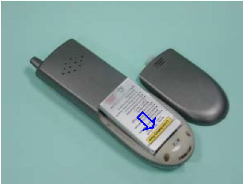
Figure 2.2 Installing or removing the Battery
