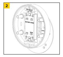
Align Housing Assembly onto Mounting Keys and slide down until Locking Tab engages. To remove, press Locking Tab and slide up.
