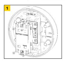
Remove four (4) screws on Battery Enclosure.
