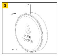
Insert Faceplate into Housing Assembly and use Hex Key to engage spring clips on the top and bottom of Housing Assembly. To remove, use Hex Key to disengage spring clips.
