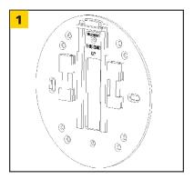
Install Mounting Bracket using at least two (2) #8 countersunk head screws. Any mounting holes may be used. Observe "THIS END UP".
