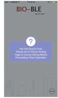
A hint to access into the phone setting page (not the App device page) - Bluetooth - to find the lock in the paired phone list, and click to cancel the pairing.
