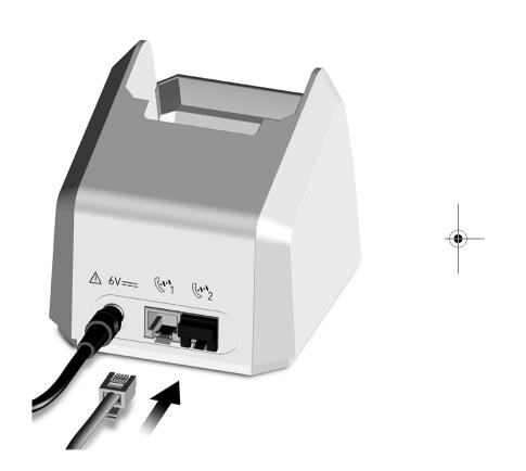
Now insert the free end of your telephone cable into the inlet of the charging station.
