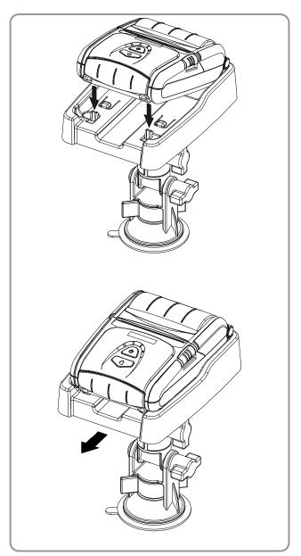
1) Insert the printer as shown in the figure on the left, and then press it in the direction of the arrows.
