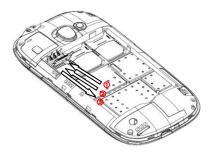
1 Hold down the microSD sheet , let go , iron spring. 2 microSD card inserted into the card slot
