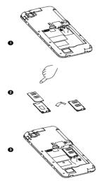
3. Finally insert the SIM card tray back to the mobile phone , and then insert the battery and replace the rear cover of the mobile phone.
