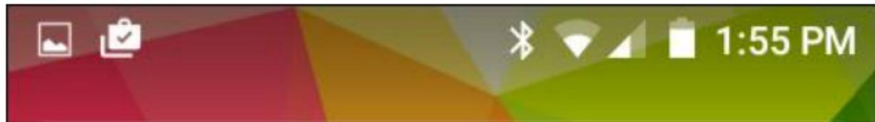
On the notification bar, several icons will appear such as network signal bar, battery indicator, data indicator, Bluetooth, and Wi-Fi. You may slide the notification bar down with your finger to display any pending notifications or actions.
