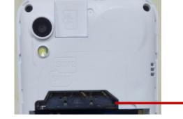
SIM Card Slot (Place the SIM card on top of the tray)
