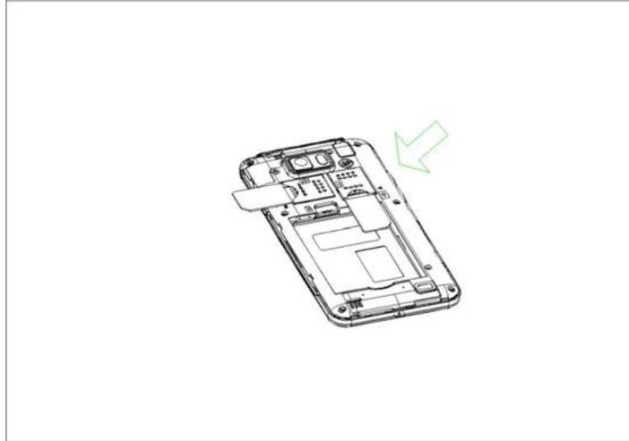
3. Finally insert the battery and replace the rear cover of the mobile phone.
