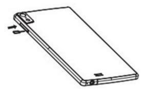
2. Insert the Micro-SIM card correctly in Micro-SIM Box.
