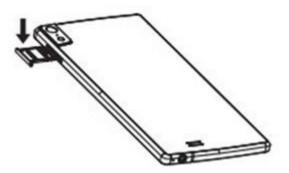
3. Push the Micro-SIM Box into the card slot.
