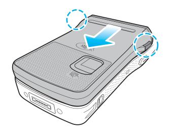
To remove, press the Finger scan remove button and slide it downwards.
