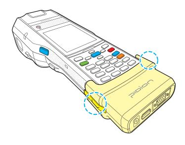
Press the remove buttons and slide it downwards to remove.
