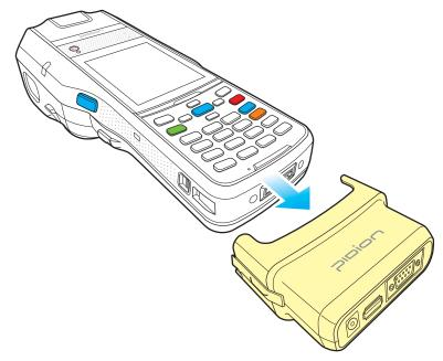
Slide the snap on in the arrow direction to install.
