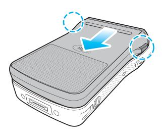
To remove, press the remove button and slide it downwards.
