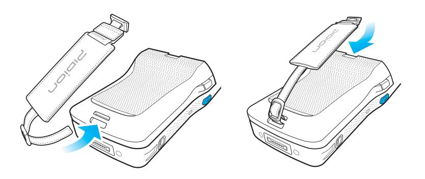
Connect the hand-strap on the battery cover's hand-strap holder.
