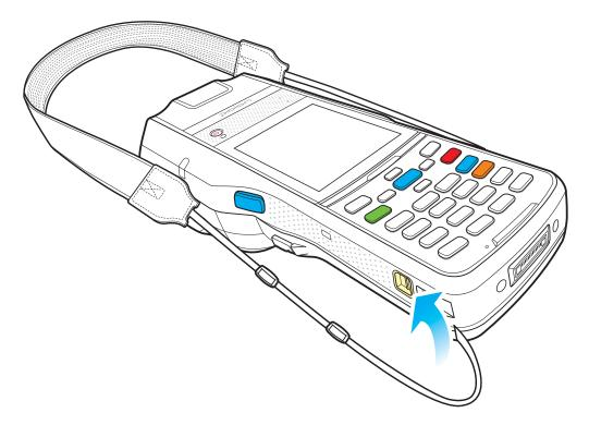
Connect the shoulder strap on both sides of the device's Shoulder strap holder.
