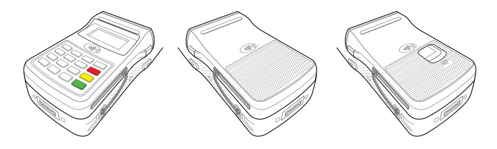
Install the IC card cover in the PINPAD/ Payment equipment / Finger scan/ IC card slot. Connect the IC card cover strap on the shoulder strap holder.
