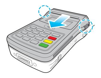
To remove, press the [PINPAD remove button] to slide the PINPAD out in the arrow direction.
