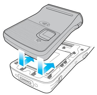
Install the Finger scan in the arrow direction.
