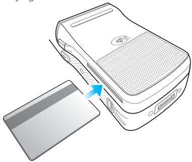
Insert with the card with the IC chip going in first. Please make sure to insert the card all the way.
