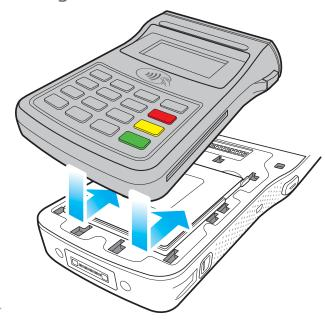
Install the PINPAD in the direction of the arrows.
