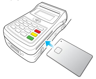
Insert with the card with the IC chip going in first. Please make sure to insert the card all the way.
