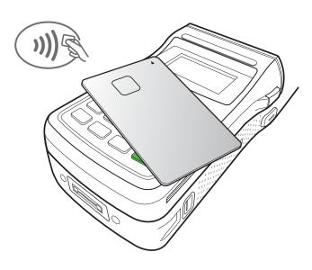
Make sure you place the card on the RFID antenna.
