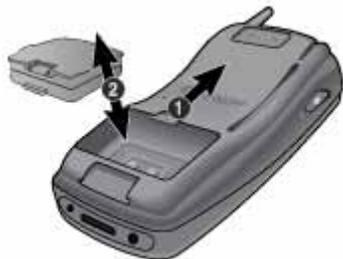
**To connect the battery:** depress the Battery Connect/Disconnect button and gently push the battery in until it clicks into place.
