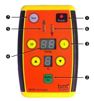
(transmit) LEDs **5** will illuminate briefly. Activation is more reliable if the *Activator* is pointing down at the BMM® (approx. 45°) as shown in the photo in Section 2.1.
