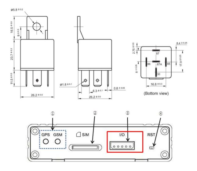
Connect the pin number 85 of relay in the below picture with the number 4 of ③ I/O connector in the above picture. And connect the pin number 30 and 86 of relay with the battery + terminal (12V or 24V). Connect 87A pin of the relay to the power source of car fuel pump. For a car ignition interlock, it interrupts the power of the fuel pump system to prevent ignition.
