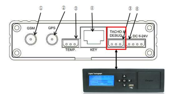
When you install the digital tachograph, refer to the "Instruction manual of digital tachograph"
