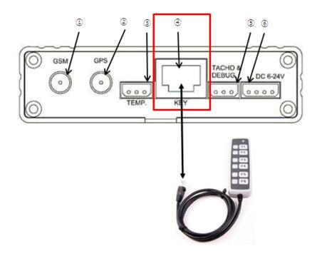
You can use F1 to F5 in the keypad. If you push each button, its applicable information is transmitted to the server. Functions in the keypad may be changed depending on the operating company. For example: F1 – car departure, F2 – cargo loading finish, F3 – cargo unloading finish, F4 – car arrival. If you push the Key among F1 ~ F5, the LED in the keypad blinks and the LED in the keypad stays on during the transmission to the server. If transmission to the server is completed, the LED gets off.
