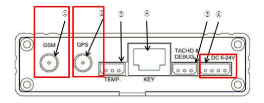
(2) Connect the power cable with ⑥ DC 6-24V connector in the above picture. Connect Cable 1 with the car battery + terminal (12V or 24V), and connect Cable 2 with the power inlet (cigar jack or radio power socket) after turning on the car ignition key, or connect this with IGN1(IGNITION 1), IGN2(IGNITION 2), or ACC pin according to the car manual. Connect Cable 3 & 4 with the car battery – terminal(Ground).
