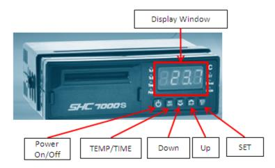
(3) If you continue to press the Temperature/time button of thermograph, the contents in the display window of thermograph appears in the following sequence.
