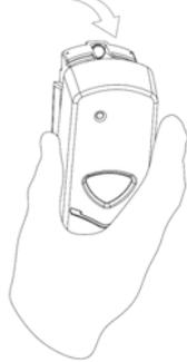
**Note:** DO NOT use a screw driver or other implement to remove cover. Incorrect removal of cover may damage the LED and void the warranty.
