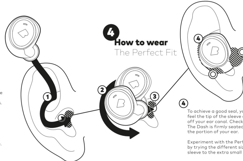
To achieve a good seal, you should feel the tip of the sleeve close off your ear canal. Check that The Dash is firmly seated within the portion of your ear.
