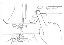
2. While holding the upper thread, press the needle position button to raise the needle.
