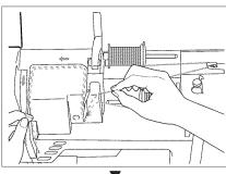
7. Set the thread around the thread guide plate, then pass the thread through the groove according to threading sequence (numbers) indicated on the machine.
