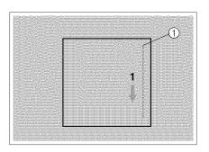
3. Set the needle in the fabric at the sewing start point, and sew seam "1" as shown.
