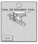
This message is displayed when the buttonhole lever is up, a buttonhole stitch is selected, and the "Start/ Stop" button or "Reverse/Reinforcement Stitch" button is pushed.
