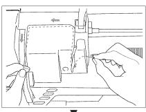
6. Pass the thread through the groove according to the threading sequence (numbers) indicated on the machine.
