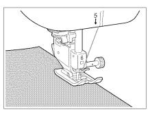
2. Attach presser foot "N". Sew scallop stitches along the edge of the fabric. Do not sew directly on the edge of the fabric.
