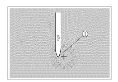
3. Attach monogramming foot "N", then turn the balance wheel to check the needle drop position. Lower the presser foot lever and start sewing. When sewing is finished, the machine sews reinforcement stitches and stops automatically.
