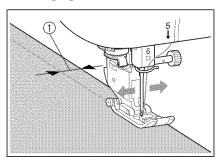
When you select left needle position stitch patterns, you can use — and + in the Stitch Width display to change the position of the needle. Match the distance from the right edge of the presser foot to the needle with the stitch width, then align the edge of the presser foot with the edge of the fabric during sewing for an attractive finish.
