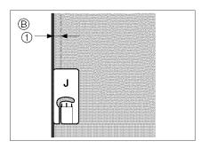
(B) To align a 6.5 mm (1/4 inch) seam allowance with the left edge of the presser foot.
