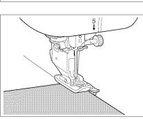
2. Attach presser foot "G". Lower the presser foot so that the presser foot guide is exactly against the edge of the fabric.
