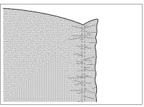
2. Sew 2 rows of straight stitches on the right side of the fabric, then pull the bobbin thread to gain the necessary gather.
