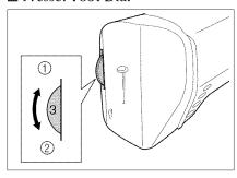
Turn the presser foot dial in order to adjust the pressure applied by the presser foot. The higher the number, the stronger the pressure will be. The presser foot dial has settings from 1 (weakest) to 4 (strongest). Use setting "3" for normal sewing. Lower the presser foot lever before turning the presser foot dial. If you adjust the setting, be sure to return it to "3" after sewing.
