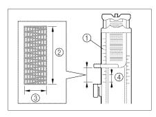
2. Attach buttonhole foot "A" and set the scale to the desired length of the darning.
