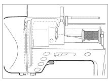
2. Do the upper threading. Follow the steps for threading a single needle for the first threading (see page 1-32 "Upper Threading").
