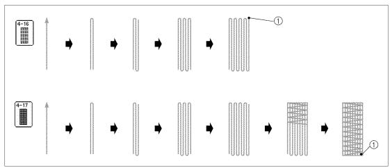
① Cycle of reinforcement stitches
