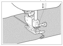
Turn back the desired width of fabric and position it over the lower fabric, then sew so that the stitch bridges both pieces of fabric.
