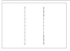
Reverse/reinforcement stitches are generally necessary at the beginning and end of sewing. You can use "Reverse/ Reinforcement Stitch" button to sew reverse/reinforcement stitches manually (see page 1-4).
