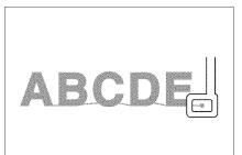
8. Use the arrow keys to move the needle to the position where the previous pattern stopped.
