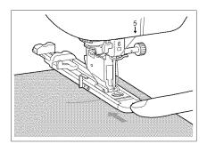
3. Check that the needle drops at the desired position and lower the presser foot lever, making sure the upper thread passes underneath the buttonhole foot.
