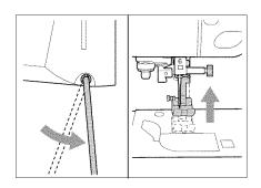
Use your knee to move the knee lifter to the right in order to raise the presser foot. Release to the left for the presser foot to lower.
