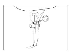
8. Do not set the thread in the needle clamp thread guide on the needle bar. Thread the needle on the right side.
