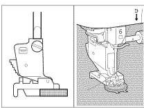
3. Attach button sewing foot "M", place the button in the presser foot, and lower the presser foot lever.
