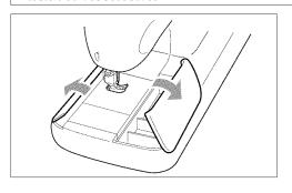
Pull the top of the flat-bed attachment towards you to open the accessory compartment.
