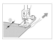
When edge stitching a short stitch length and close to the edge of the fabric, the presser foot may not cover enough fabric for proper feeding. Before you begin to sew, sew a basting thread at the corner point. When you change direction at the corner, start sewing as you pull the basting thread toward the back.
