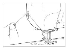
10. Use the thread cutter on the side of the machine to cut the thread.
