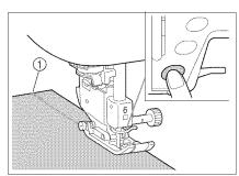
3. Set the fabric in the start position and start sewing. The machine will automatically sew reverse stitches (or reinforcement stitches) and then continue sewing.
