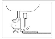
The sewing machine can sew fabrics up to 6 mm(1/4 inch) thick. If the thickness of a seam causes sewing to occur on an angle, help guide the fabric by hand and sew on the downward slope.
