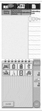
2. The machine displays the patterns saved in the memory. Select a pattern to retrieve.
