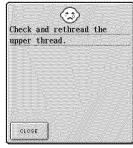
This message is displayed when the upper thread is broken or not threaded correctly, and the "Start/Stop" button or the "Reverse/ Reinforcement Stitch" button is pressed.
