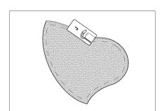
5. Use the quilting appliqué stitch to attach the appliqué. Sew around the edge, while dropping the needle as close to the edge as possible.
