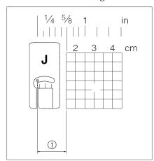
For standard 16 mm (5/8 inch) seam allowance, set width on LCD.
