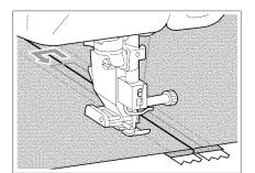
5. Topstitch 7 to 10 mm (1/4 to 3/8 inch) from the seamed edge of the fabric, then remove the basting.
