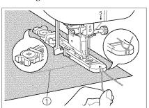
When sewing on stretch fabric with buttonhole stitches over a gimp thread.
