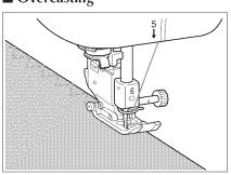
Use this stitch to sew overcasting on the edge of stretch fabrics. Sew the overcasting along the edge of the fabric with the needle dropping off the edge of the fabric at the right.
