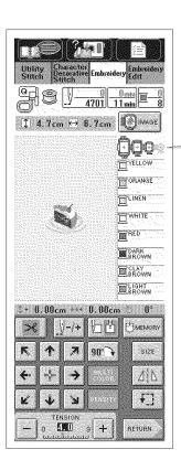
Select a frame that matches the pattern size. Frame options are displayed on the LCD.
