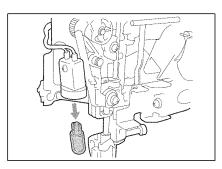
3. Remove the light bulb as shown, and align the projection on the light bulb with the notch in the socket. Replace it with a new light bulb.
