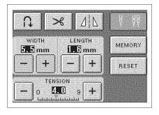
To change the needle position use + or - in the width display.
