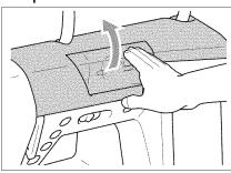
Open the top cover to wind the bobbin or do the upper threading. To open the cover, place your hand under the clear section of the cover and lift up.
