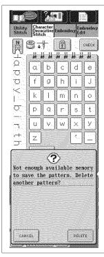
If you see this screen after pressing [ the machine's memory], the machine's memory is full and can not save the currently selected stitch pattern. To save the stitch pattern in the machine's memory, you have to delete a previously saved stitch pattern.
