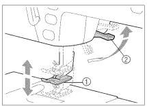
Lower the presser foot lever to lower the presser foot and apply pressure to the fabric. If the presser foot is raised to the second position, and you want to sew heavy weight, stacked fabrics, etc., that are hard to set under the presser foot, raise the presser foot lever higher and hold it to make room for the fabric (see page 2-4).
