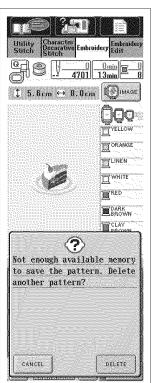
If the screen at left displays, the maximum number of patterns have been saved, or the pattern you want to save takes a lot of memory, and the machine can not save it. If you delete a previously saved pattern, you can save the current pattern.
