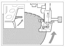
Stop the machine with the needle in the fabric outside the appliqué. Raise the presser foot and turn the fabric a little bit at a time while sewing, for an attractive finish to the seam.
