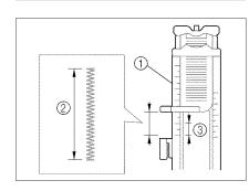
2. Attach buttonhole foot "A" and set the scale to the length of the bar tack you wish to sew.
