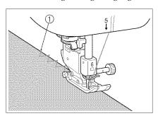
Sew the overcasting along the edge of the fabric so that the right-hand side needle drop point is over the edge of the fabric.
