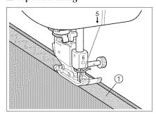
Stretch the tape flat. While stretching the tape flat, sew the tape to the fabric.
