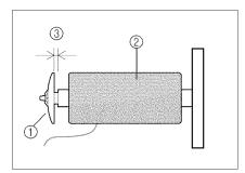
When sewing with fine, cross-wound thread (see the illustration), use the small spool cap, and leave a small space between the cap and the thread spool (see the illustration at left).
