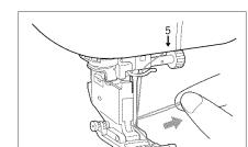
14. Pull the thread loop toward the back of the machine.
