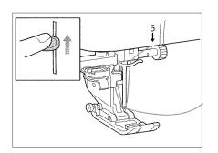
13. Slowly return the needle threader lever to its original position. Check that the hook has pulled the thread through the eye, then release the lever.
