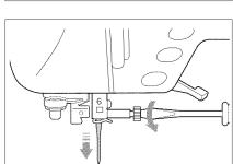
Use the screwdriver to turn the screw toward the front of the machine and loosen the screw, then remove the needle.
