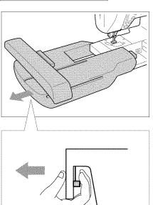
2. Turn off the main power switch. Hold the back left side of the embroidery unit. Hold down the release button, and pull the embroidery unit away from the machine as shown.
