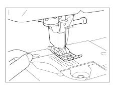
3. Gently pull the upper thread, and a loop of the bobbin thread will come out of the hole in the needle plate.
