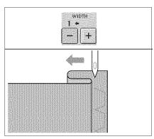
Adjust the width so that the needle slightly catches the fold by pressing — in the WIDTH display.
