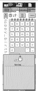
3. The screen at left will display. The machine will automatically save the stitch pattern and return to the original screen.
