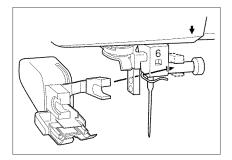
6. Set the operation lever of the walking foot so that the fork surrounds the needle clamp, and set the walking foot on the presser foot shaft.
