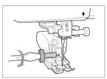
7. Lower the presser foot lever, insert the screw (large) for the walking foot, and tighten the screw securely with the screwdriver.
