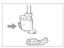
3. Press the black button on the presser foot holder, and remove the presser foot.
