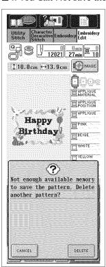
If the screen shown at left displays, the maximum number of patterns have been saved, or the pattern you want to save takes a lot of memory, the machine can not save it. If you delete a previously saved pattern, you can save the current pattern.
