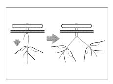
5. From the wrong side of the fabric, pull the end of the bobbin thread to pull the upper thread through to the wrong side of the fabric. Tie the two thread ends together and cut the threads.
