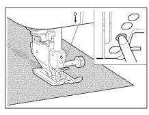
5. Press the "Start/Stop" button to stop sewing, then press the "Reverse/Reinforcement Stitch" button to sew reinforcement stitches.
