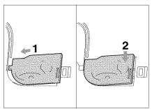
5. Replace the bobbin cover. Place the left tab in place (see arrow 1 at left), then press lightly on the right side (see arrow 2 at left) until the cover clicks into place.
