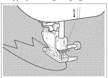
Attach the appliqué using a temporary spray adhesive or basting, then sew it.
