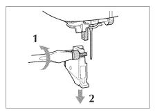
4. Loosen the screw of the presser foot holder to remove the presser foot holder.
