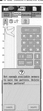
If the screen shown at the left appears after the machine's memory is full or the stitch pattern being saved is larger than the amount of space available in the memory. To be able to save the stitch pattern in the machine's memory, a previously saved stitch pattern must be deleted.
