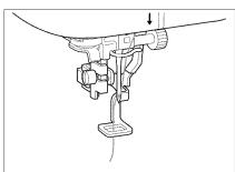
1. Thread the machine with the first color, and pass the end of the thread through the hole in embroidery foot "Q".
