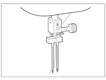
3. Pass the thread through the needle clamp thread guide on the needle bar, then thread the needle on the left side.
