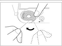
3. Put the bobbin in the shuttle, making sure the thread unrolls as shown.
