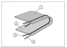
The upper and lower threads should cross near the center of the fabric. If thread tension is not properly set, the seam may have a poor finish or the fabric may pucker.
