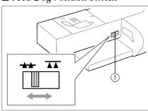
Use this switch when attaching buttons (see page 3-61) or for other similar projects. Remove the flat bed attachment and raise the presser foot lever to operate the feed dog position switch. Set the lever in the \*\*position for normal sewing
