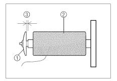
When sewing with fine, cross-wound thread (see the illustration at left), use the small spool cap, and leave a small space between the cap and the thread spool (see the illustration at left).
