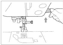
If the presser foot lever is in the up position, and you are sewing heavyweight or multiple layers of fabric which does not fit easily under the presser foot, raise the presser foot lever as high as possible by hand to bring the presser foot to its highest position. The fabric will now fit under the presser foot.
