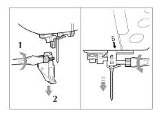
1. Turn off the power. Remove the presser foot holder and the needle.
