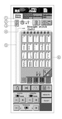
① Shows the amount of thread remaining in the bobbin during sewing. If the display is yellow, the bobbin is running out of thread.
