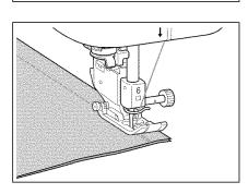
4. When sewing is completed, hold the "Reverse/Reinforcement Stitch" button to sew 3-4 reverse stitches (or reinforcement stitches) at the end of seam.
