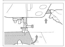
Stop the machine. Leave the needle in the fabric, and raise the presser foot. Using the needle as a pivot, turn the fabric so that you can sew in the new direction. Lower the presser foot lever and start sewing.
