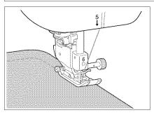
Sew slowly while keeping the seam parallel with the fabric edge as you guide the fabric around the curve.
