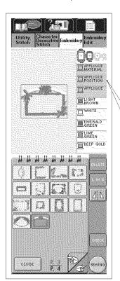
When sewing an embroidery pattern with an appliqué, the color sewing order display shows "Appliqué Material," "Appliqué Position," "Appliqué", and then the sewing order of the colors around the appliqué.
