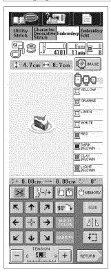
Use the arrow keys to move the pattern in the direction shown
