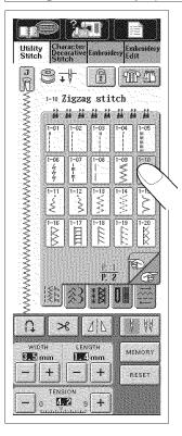
Press a key with your finger to select the stitch pattern, or to select a machine function, or operation indicated on the key.
