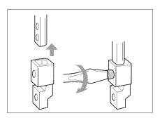
5. Set the low shank adapter for the walking foot that came with your machine on the presser foot shaft, and push it up as far as possible. Tighten the screw securely with the screwdriver.
