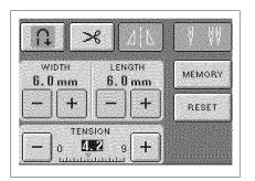
2. Use | - | + | in either the stitch width display or the stitch length display to choose the size of the eyelet. Large 7 mm (1/4 inch), Medium 6 mm (15/64 inch), Small 5 mm (3/16 inch) actual size.
