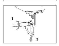
4. Use the included screwdriver to loosen the screw of the presser foot holder, then remove the presser foot holder.
