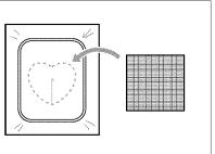
2. Place the appliqué fabric over the pattern embroidered in step 1. Be sure that the appliqué fabric completely covers the seam.
