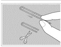
Once sewing is completed, gently pull the gimp thread to remove any slack, and trim off any excess.
