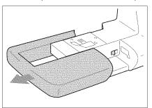
1. Remove the flat bed attachment to create the free arm function.
