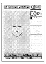
1. Select a straight stitch frame pattern. Embroider the pattern onto the appliqué material, then cut neatly around the outside of the shape.
