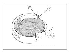
3. Turn the balance wheel, and align the notch of shuttle a little to the left of the shelf of race, as shown.
