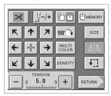
The upper thread will become loose. The embroidery thread on the right side of the fabric will loosen, the thread locks may loosen, or loops may appear on the right side of the fabric.
