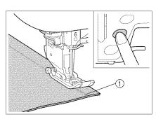
4. Press the "Reverse/Reinforcement Stitching" button. The machine will sew reverse stitches (or reinforcement stitches), then trim the thread.
