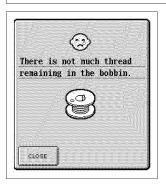
When the bobbin begins to run out of thread during sewing, the message shown at left will display. If the pattern is nearly complete at this time, you can finish the pattern safely without changing the bobbin thread. If there is a large portion of the pattern left to finish, it is recommended to change the bobbin thread before continuing. If the message at left displays, follow the steps below.
