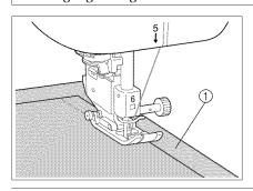
Place thin paper under thin fabrics to make sewing easier. Gently tear off the paper or the stabilizer for embroidery after sewing.
