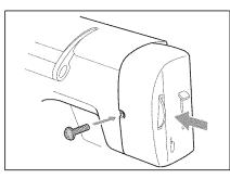
4. Place light cover and tighten the screw on the back of the machine.
