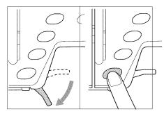
6. Lower the presser foot lever, and press the "Start/Stop" button to continue sewing.
