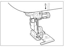
5. Slowly lower the presser foot lever, and then position the pin on the presser foot (side cutter) in the notch of the presser foot holder to attach the presser foot (side cutter).
