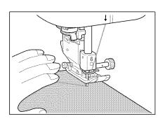
2. Attach presser foot "J". Hold the thread tails and fabric with your left hand, and turn the balance wheel with your right hand to insert the needle into the fabric. This is the sewing start position.
