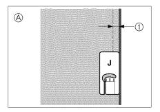
(A) To align a 6.5 mm (1/4 inch) seam allowance with the right edge of the presser foot.
