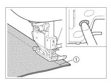
4. Press the "Reverse/Reinforcement Stitch" button. The machine will sew reverse stitches (or reinforcement stitches) and stop.
