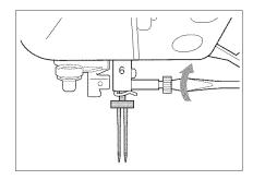
1. Turn the main power switch to OFF, and install the twin needle (see page 1-43 "Changing the Needle").
