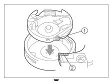
6. Check that the notch on the shuttle is in the same position as when you removed the race. Position the race so that the shelf and spring are aligned, and insert the race.
