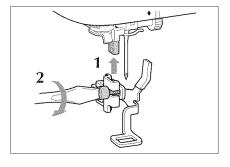
5. Set embroidery foot "Q" on the presser foot bar so that the arm of embroidery foot "Q" is in contact with the back of the needle holder, then use the included screwdriver to firmly tighten the screw.
