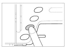
2. Attach presser foot "J". Press the "Reverse/ Reinforcement Stitch" button to sew reinforcement stitches, then continue sewing.
