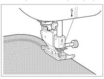
Shorten the stitch length setting to obtain a fine stitch. Sew slowly, keeping the seams parallel with the fabric edge as you guide the fabric around the curve.
