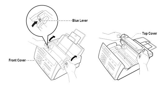
Pull the jammed paper gently from the paper feeder toward the back of the fax machine. If the paper remains jammed, then pull it toward the front of the machine.
