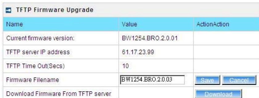
Figure 130 – TFTP Firmware Upgrade setting
