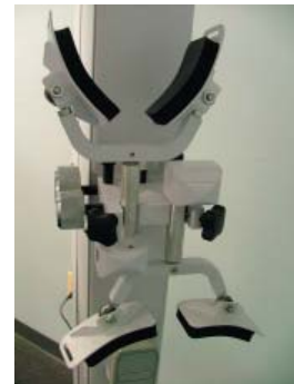
Figure 1-6. Head Braces Secured to Column
