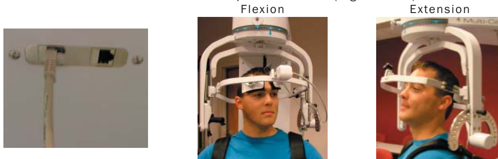
Figure 6-56. MCU™ RJ45 Jack and Final 25° Isometric Flexion & Extension Set-ups
