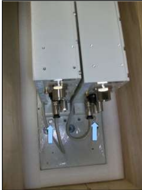
Figure 4-4. Remove the two M8 Fasteners
