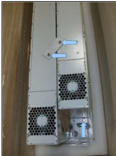
Figure 4-5. Remove the M8 Fastener and the two M5 Fasteners
