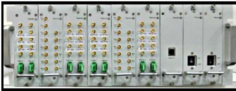
Figure 3-2. Host Unit Multiple-Slot Assembly
