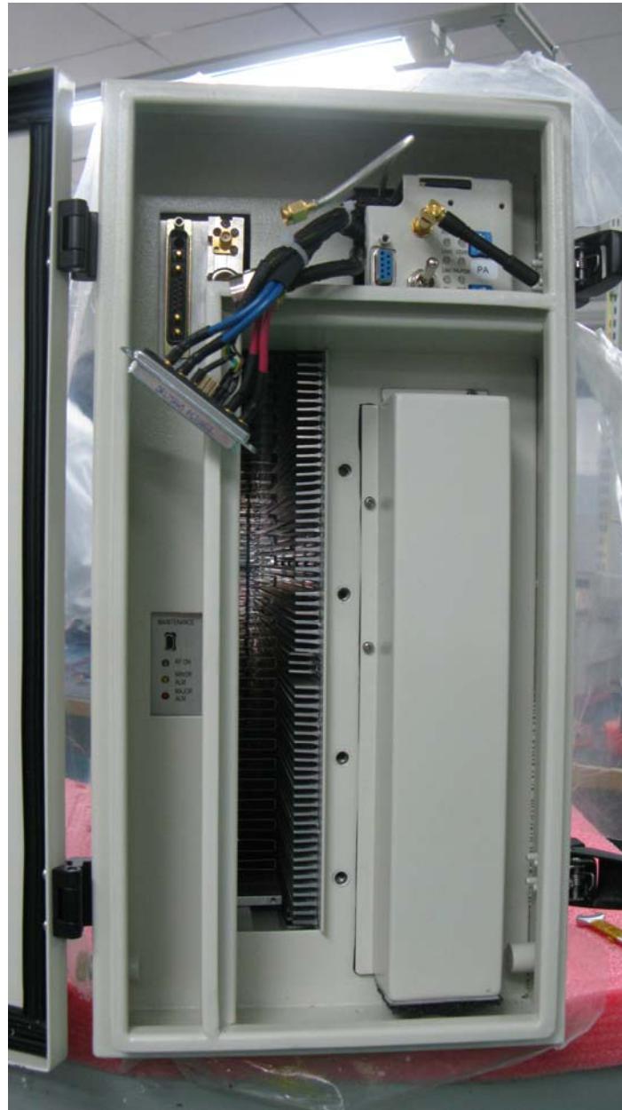
Figure 6 the rear side of an assembled LPA1900
