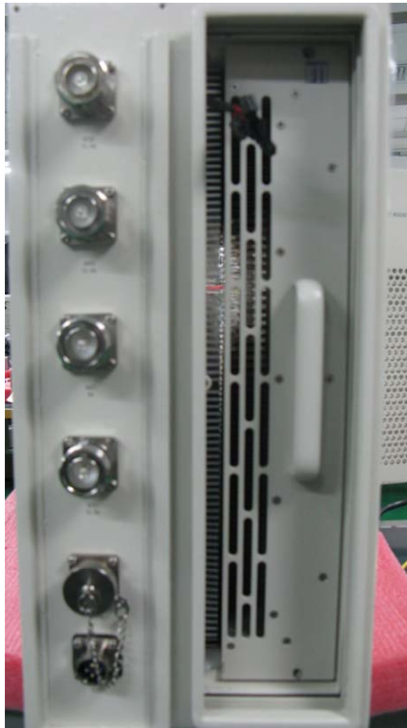
Figure 5 the front side of an assembled LPA1900
