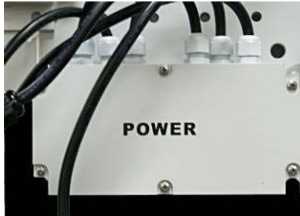
Figure 35 AC Power Junction Box
