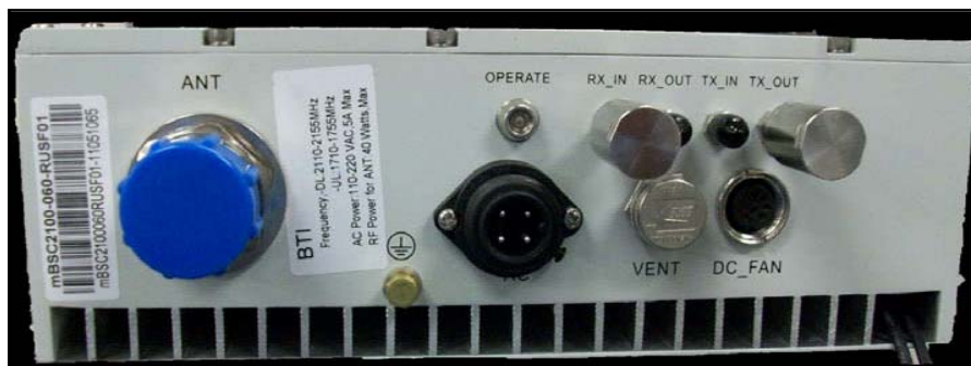
Figure 3-9. User Interface of SLAVE Remote Unit
