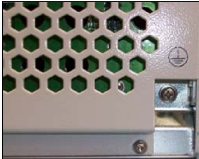
Figure 4-15. Host Unit Grounding Connection
