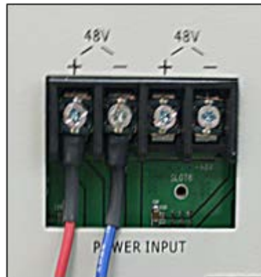
Figure 27 48VDC Host Power Connection
