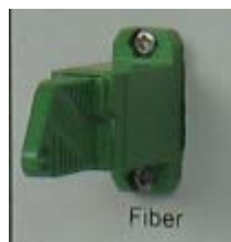
Figure 26 E2000 Fiber Optic Port on Host Unit FIU
