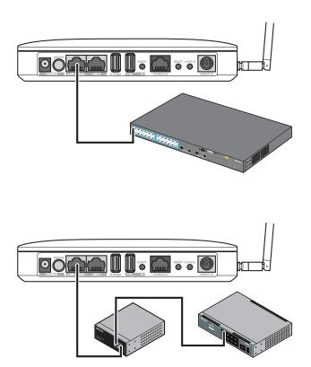
Note: Be sure that the cable connecting the AirStation and power sourcing equipment is an enhanced Category 5 or higher 4-pair cable.
