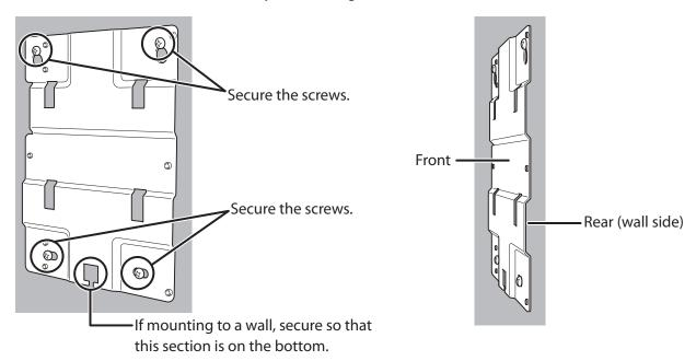
2 As shown in the figure, insert the AirStation so that it clicks into place, and then secure it in place on the wall-mounting fixture.
