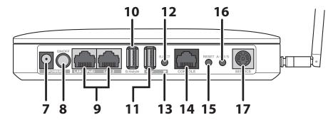
**7 DC Connector** The AC adapter (WLE-OP-AC12, sold separately) is connected here.
