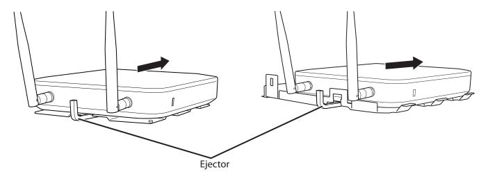
Insert the supplied ejector into the position shown in the figure so that the clips of the AirStation are raised, and then apply force in the direction of the arrow to remove.
