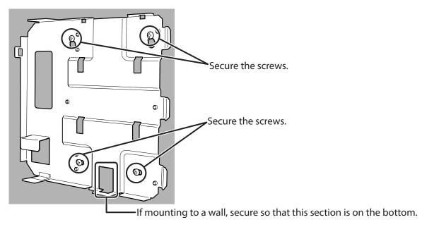
2 As shown in the figure, insert the AirStation so that it clicks into place, and then secure it on the wall-mounting fixture.
