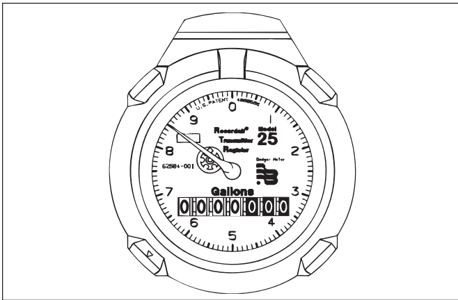
Figure 1 Identification - Recordall Transmitter Register
