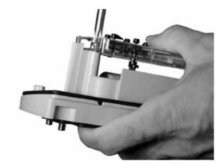
4. Test the drive pawl connection by turning the shaft on the rear of the endpoint several times. If dragging or friction is felt, reposition the index to eliminate any drag. The dials should turn smoothly.
