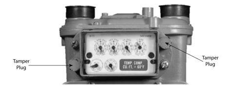
2. Use a large screwdriver to remove and discard the four (4) mounting screws and the cover.
