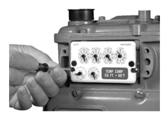
Page 8 (1-11) Shown below is an American gas meter with the tamper plugs, index and gasket removed.
