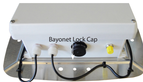
Figure 22: RJ45 Receptacle Bayonet Lock Cap (LAN with power shown)
