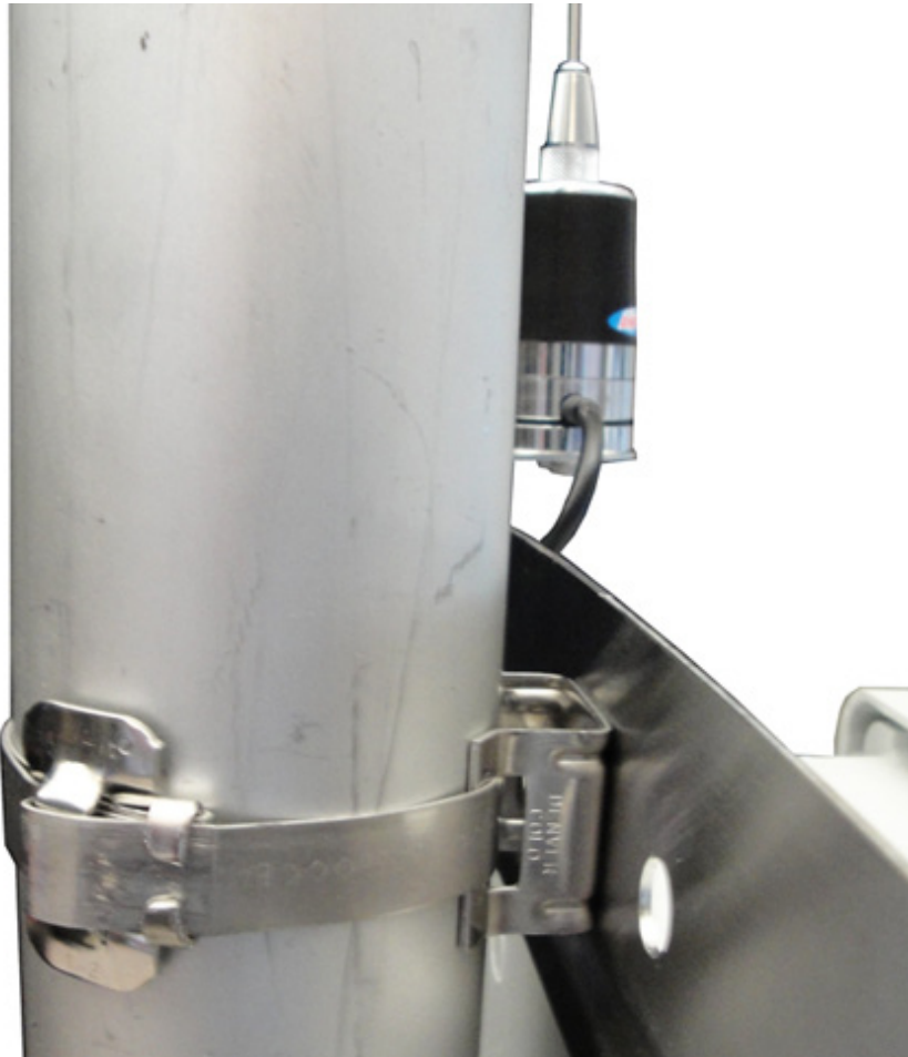
Figure 8: Network Gateway Transceiver Shown with BAND-IT Mounting Hardware
