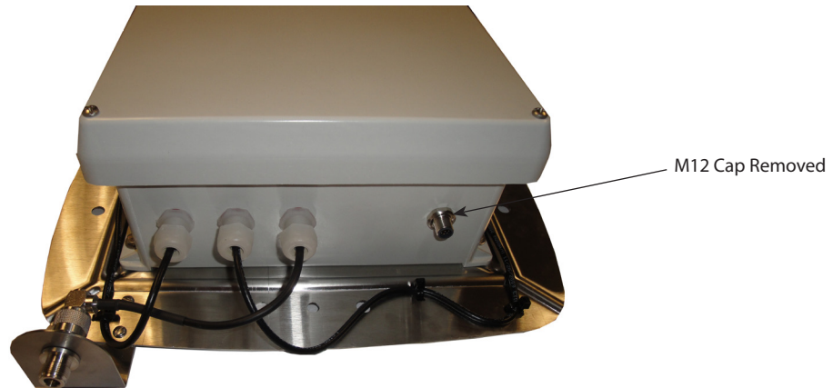
Figure 13: Bottom of Network Gateway Transceiver (GPRS unit shown)
